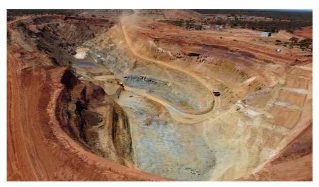
Figure 2 - View of Sand King looking north showing cut back commenced in the southern half of the open pit
