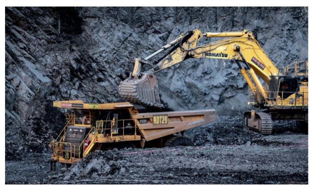
Figure 1 - Komatsu 1250 Digger loading Caterpillar 777 LHD Truck at Missouri Open Pit
